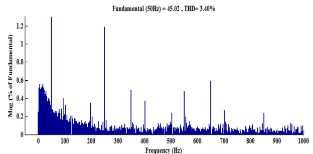
Fig. 5: Total Harmonic Distortion of Load Voltage.
