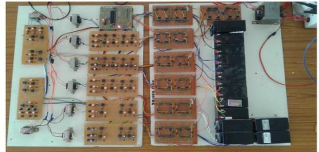
Fig. 7: Hardware Setup of Driver Circuit and Inverter Circuit.
