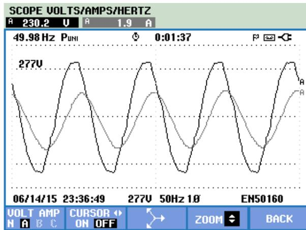
Fig. 11: Load Voltage after Voltage swell Compensation.
