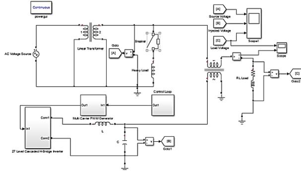
Fig. 1: Simulation Block Diagram of Single Phase DVR.
