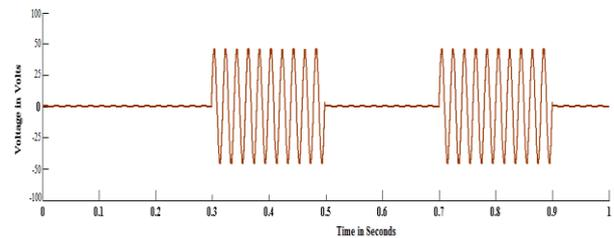
Fig. 3: Voltage Injected by DVR during Sag and Swell.
