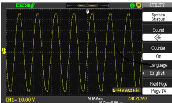
Fig. 13: Voltage Injected by DVR during Swell.
