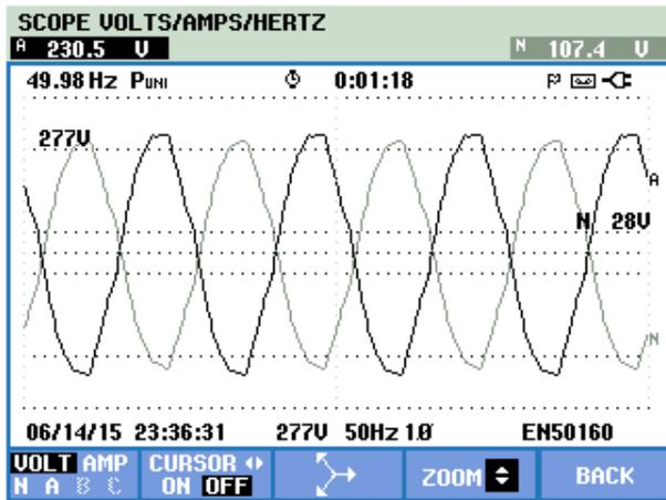
Fig. 10: Load Voltage after Voltage Sag Compensation.
