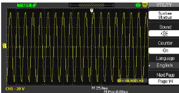
Fig. 12: Voltage Injected by DVR during Sag.
