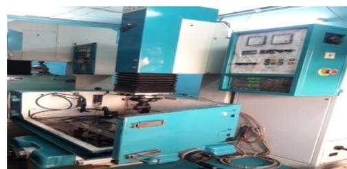
Fig. 1: Electric Discharge Machining
