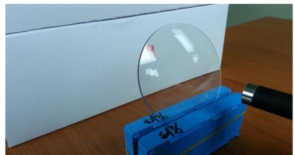
Figure 7: Purple beam cut off of UV blocking lens
