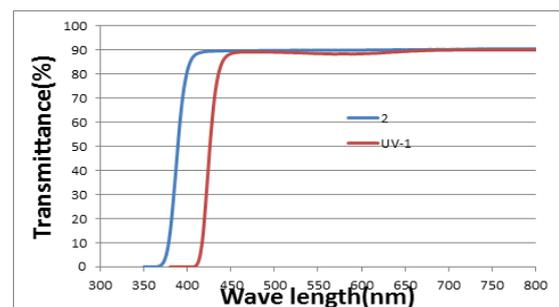
Figure 8: Comparison spectrum of 401 lens and CR39 lens
