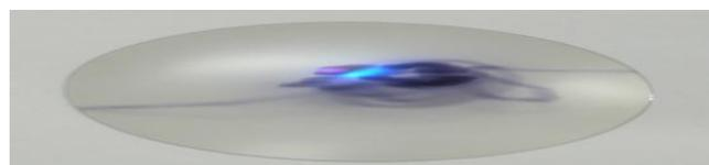
Figure 2.: Color change of a sample photochromic lens with a 405 nm laser light
