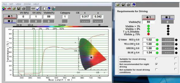
**Figure 10:** Spectrum of polarizing lens with photochromic and UV blocking
