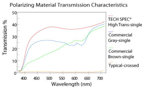
Figure 4: Transmittances of polarizing film
