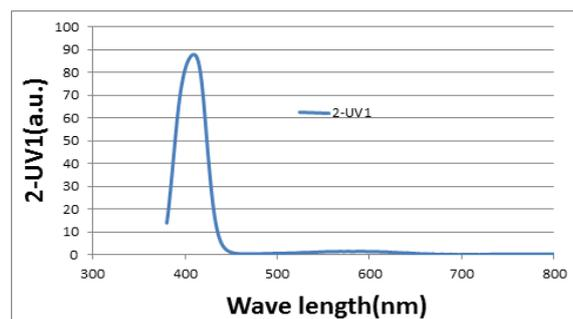
Figure 9: Difference spectrum between 401 lens and CR39 lens
