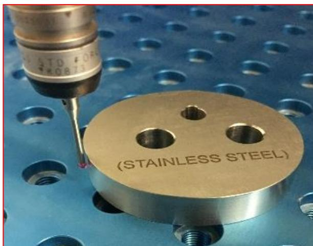
Fig. 4: Contact-Type CMM Engaged with Disc CAM.
