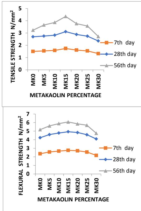
Figure 2 Variation of Tensile strength and flexural strength with metakaolin content
