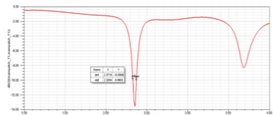
Fig. 4: Return loss of single patch antenna
