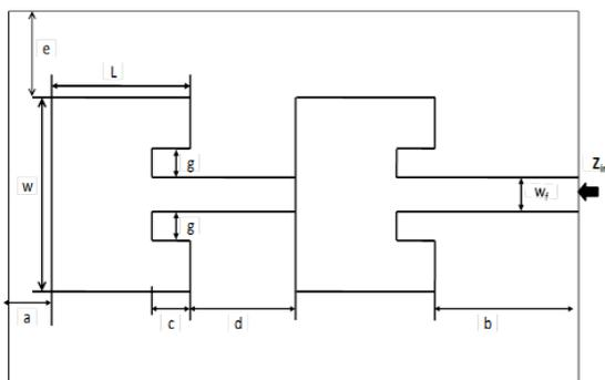
Fig. 2: Series fed microstrip patch antenna array
