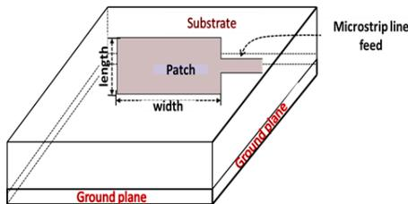
Fig. 1: Schematic diagram of Single Microstrip Patch Antenna
