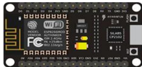
Fig. 2: NodeMCU breakout board
