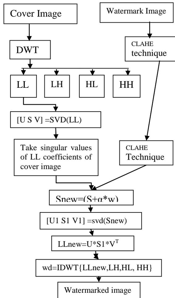
Fig. 2: Watermark embedding block diagram
