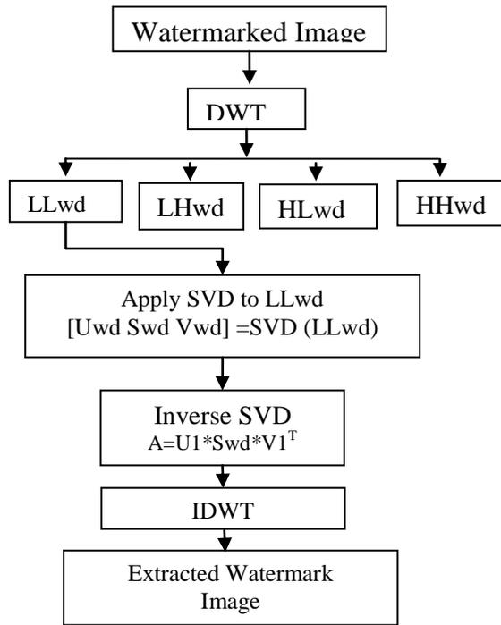
Fig. 3: Watermark extraction block diagram
