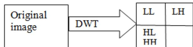
Fig. 1: DWT decomposition
