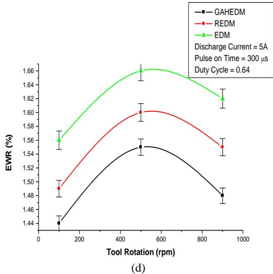
Fig. 4: Influence of (a) discharge current (b) pulse on time (c) duty cycle (d) tool rotation on EWR
