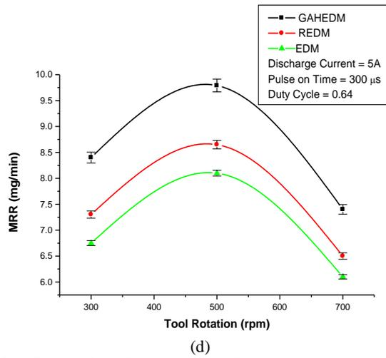
Fig. 3: Influence of (a) discharge current (b) pulse on time (c) duty cycle (d) tool rotation on MRR
