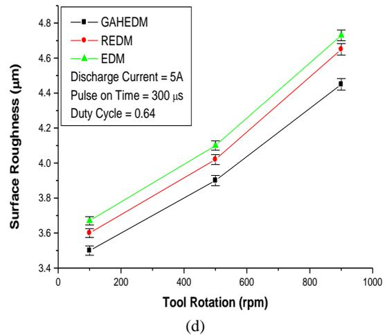
Fig. 5: Influence of (a) discharge current (b) pulse on time (c) duty cycle (d) tool rotation on SR
