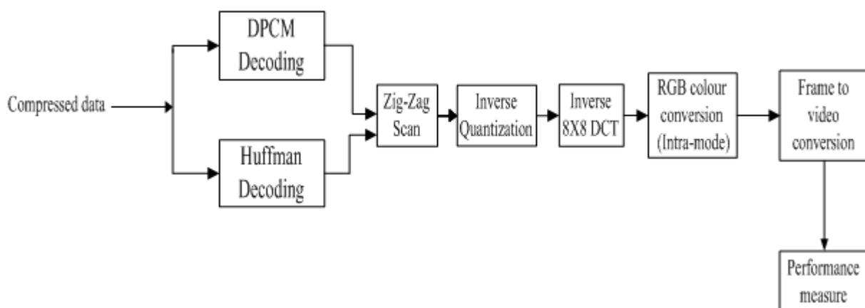
Fig. 1: Block diagram of the HSV-EPHC-IFHEVC system
