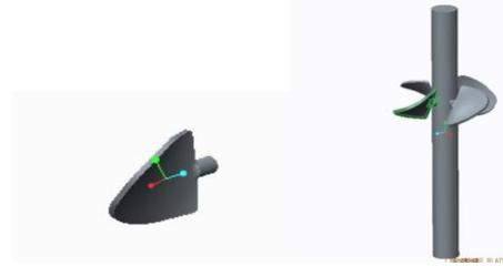
Fig. 2: Blade And Assembly View of Kaplan turbine.
