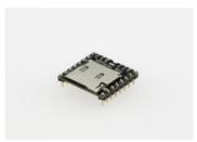
The DFPlayer Mini MP3 Player is a minor and small price MP3 module with has an simplified output directly to the speaker. The module can be used as a impartial module with involved battery, speaker and push buttons or used in combination with an Arduino UNO or any other with reception and transmission capabilities [15].
