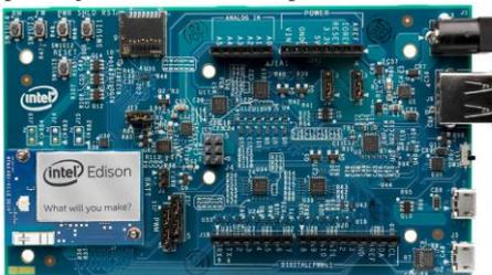
Figure 1.2: Intel Edison computing module [3]
