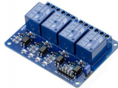
Figure 1.9: Relay module
