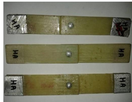
Fig. 4: Single lap hybrid (bonded-riveted) Joints –ASTM standard
