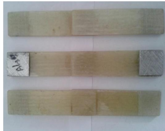
Fig. 3: Single lap Bonded Joints –ASTM standard
