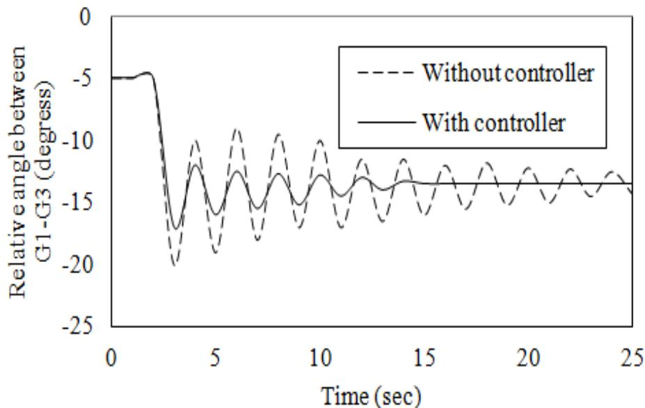
**Fig. 8:** Dynamic response of SSSC WADC during line fault at bus 20 (Relative angle between G1-G3)
