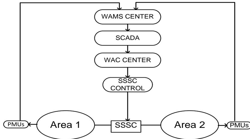
Fig. 1: Basic Wide Area Measurement (WAM) structure
