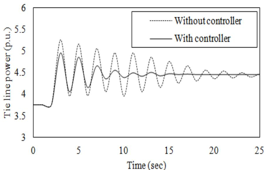
Fig. 9: Dynamic response of SSSC WADC for increased loading at bus 15
