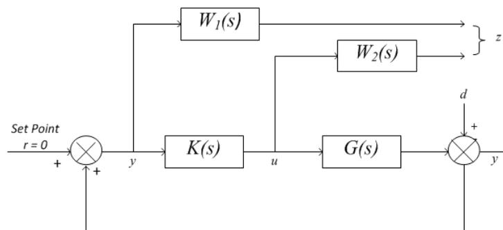
Fig. 3: Mixed sensitivity output disturbance rejection configuration
