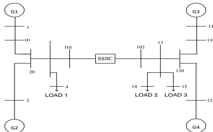
Fig. 2: Two area four machine test system
