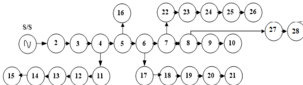
Fig. 2: One line diagram of 28-bus Indian distribution network
