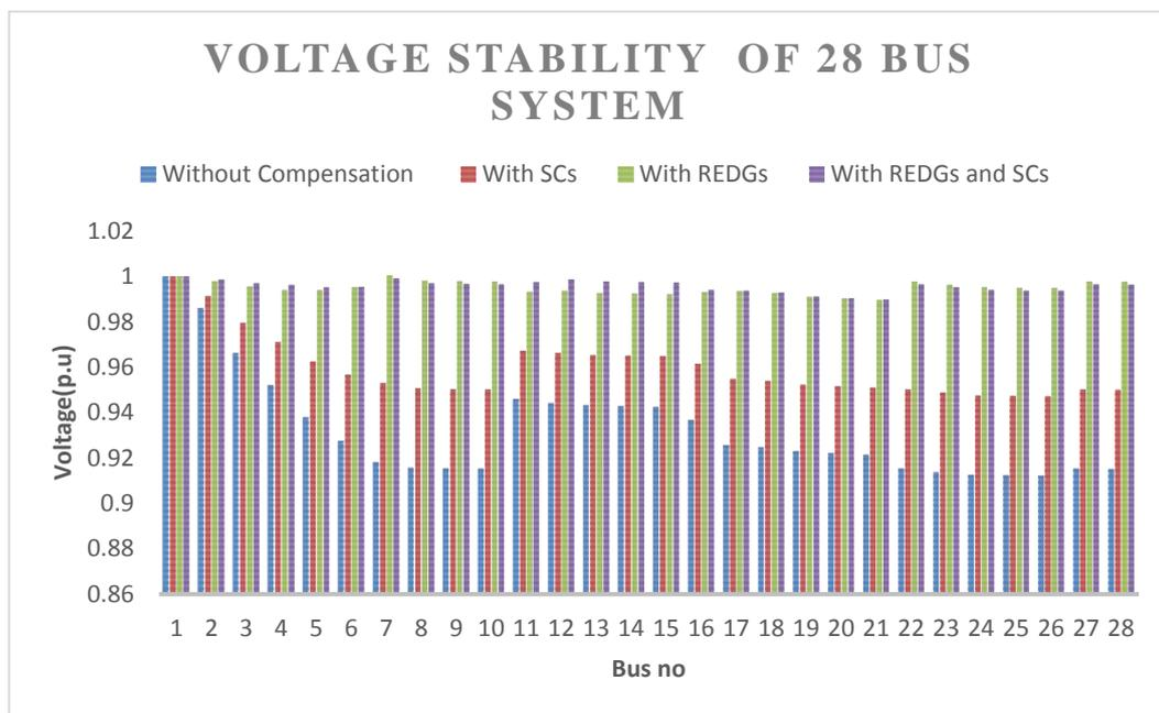
Fig. 4: Voltage stability of 28-bus Indian distribution network
