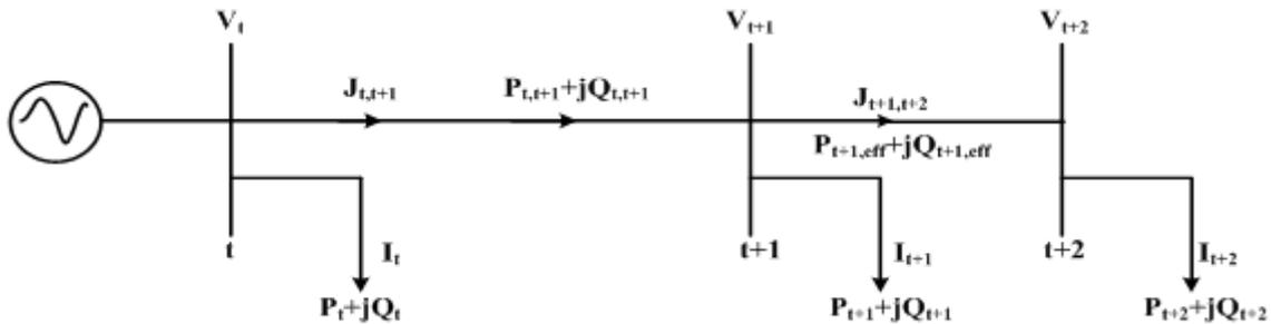
Fig. 1: Simple distribution system
