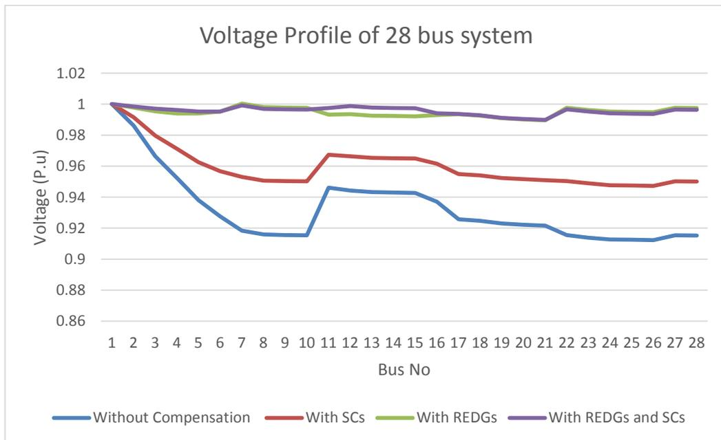
**Fig. 3:** Voltage profile of 28-bus Indian distribution network
