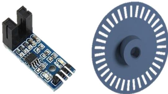
Fig. 6: (a). Infrared sensor (Left) (b). Encoder disc (Right)
