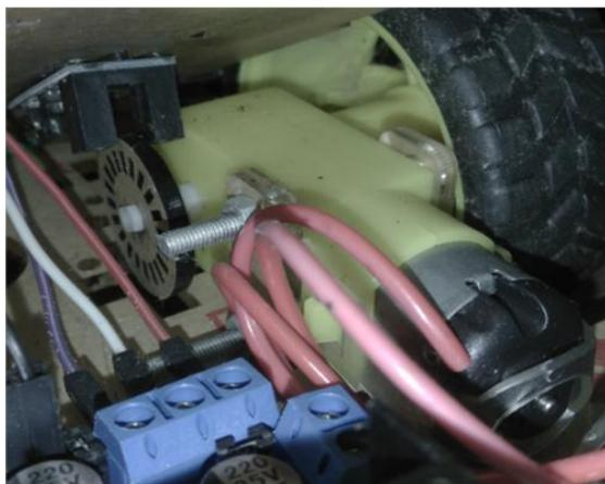
Fig. 8: Experimental smart sensor assembly setup for speed measurement
