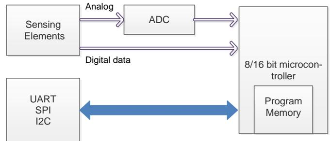
**Fig. 3:** Hardware design part for the sensor node
