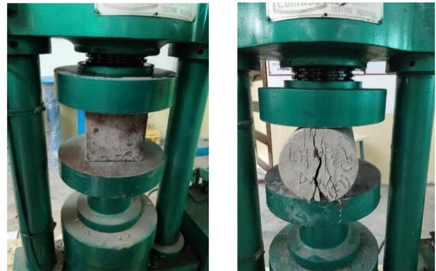
Fig. 2: Compression and Split Tensile strength testing of specimens
