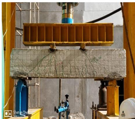
Fig. 7: Test specimen of nominal mix in SCC concrete
