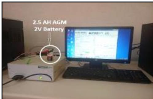
Fig. 5: Experimental test bench showing the testing device and lead-acid battery
