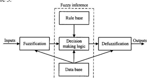
Fig. 1: Represents the block diagram of fuzzy logic
