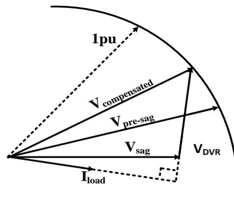
Fig. 7: In-Phase Advanced/Energy Optimization Compensation.
