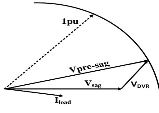
Fig. 6: Pre-Sag Injection/Compensation.
