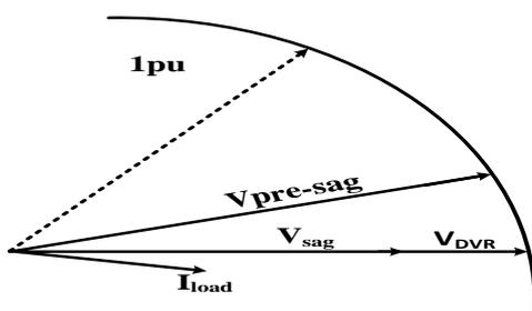
Fig. 5: In-Phase Injection/Compensation.
