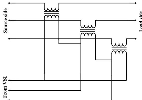
Fig. 2: Delta Open Configuration.
