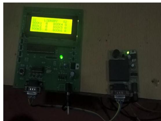
Fig. 6: Interfacing of RFID Reader with PIC Microcontroller
