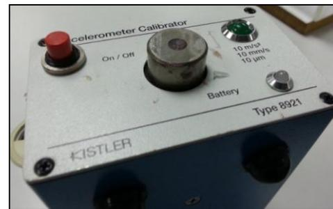
Fig. 3: The tri-axial accelerometer calibrator
