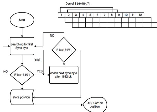
Fig. (4). Sync-byte detection process
