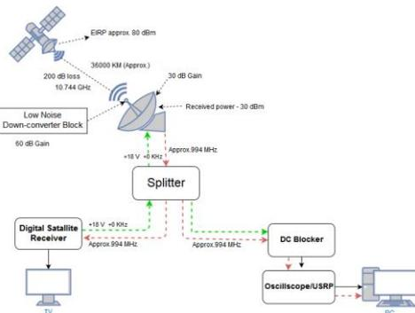
Fig. (1). Basic block diagram of satellite receiver
