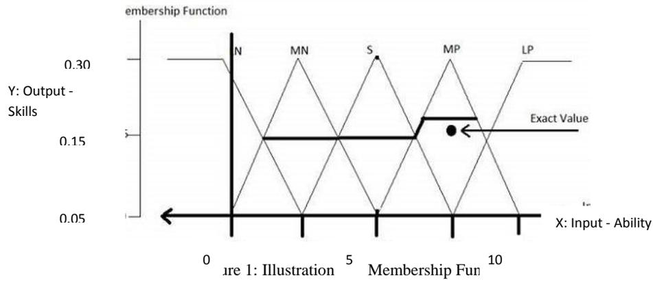
The exact value of each fuzzy output is obtained from the midpoint of the triangles of the membership function. As the input value changes, so does the output change. In this design, each child is assumed to have a maximum of 30% of the total skills in the universe of discourse and a maximum of 10 abilities to measure intelligence, which in turn determine skill.
