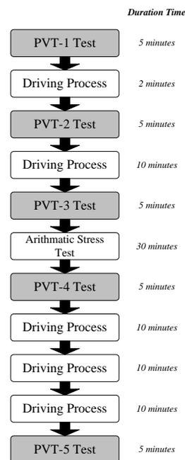
Fig. 1: Design Process of Drowsiness Detection System based on PVT Test & Arithmetic Stress Test
