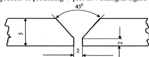
Fig 5: Plot V for welding in mm sized
