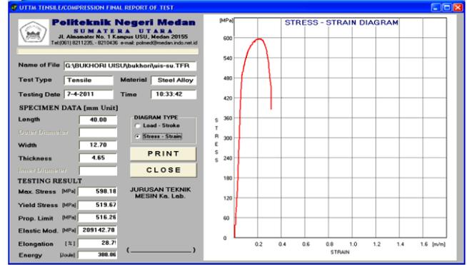
**Fig 8:** Graphic Strain Stress of raw material
