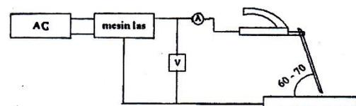
Fig 6: Set-up instrument of welding
