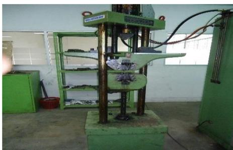
Fig 3: Universal Tensile Test Machine
