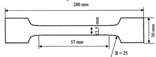
Fig 4: Specimen Tensile Test ASTM E-18
