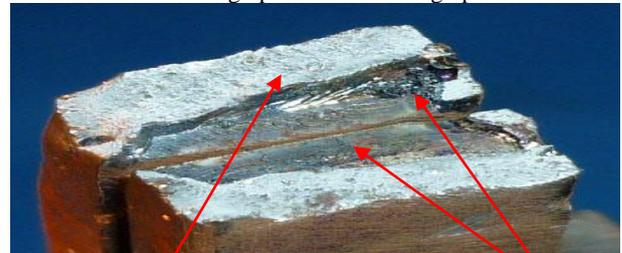
Surface of Material welding scraps      Surface Material of based plate
