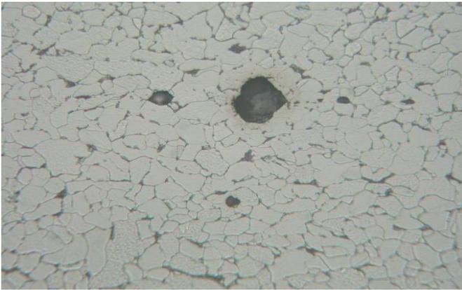
Fig 10: Structure Micro material of metal low carbon
