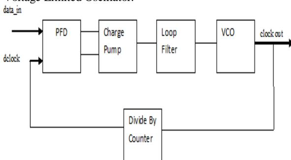
Fig. 1: Phase Locked Loop
