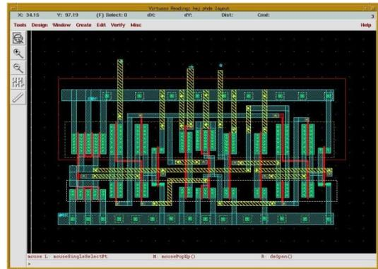
**Fig. 6:** Cell Layout of Phase Detector Circuit
