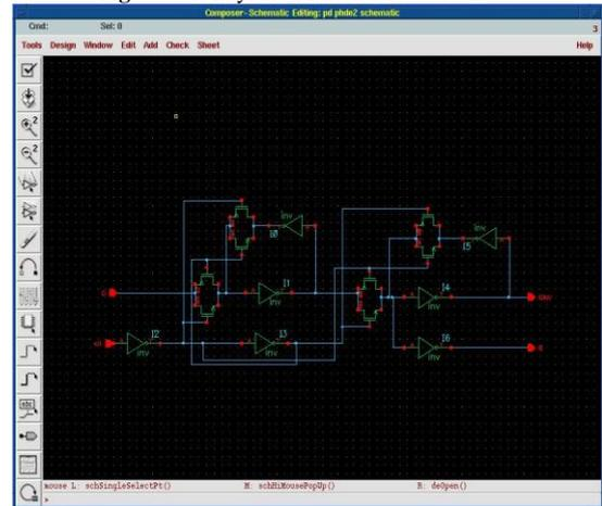
**Fig. 7:** Schematic circuit of Phase Detector
