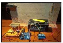
Fig. 5: Assemble Arduino, Selenoid Key, and Relay
