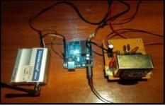
Fig. 6: Assemble SMS Gateway with Arduino
