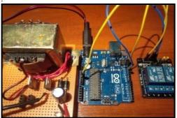
Fig. 4: Connecting Relay with Arduino Uno
