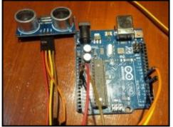
Fig. 3: Connecting Arduino Uno with Ultrasonic Sensor
