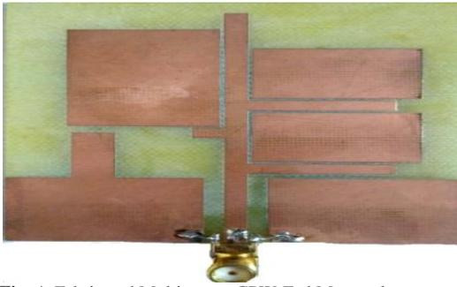
Fig. 4: Fabricated Multi-octave CPW-Fed Monopole antenna
