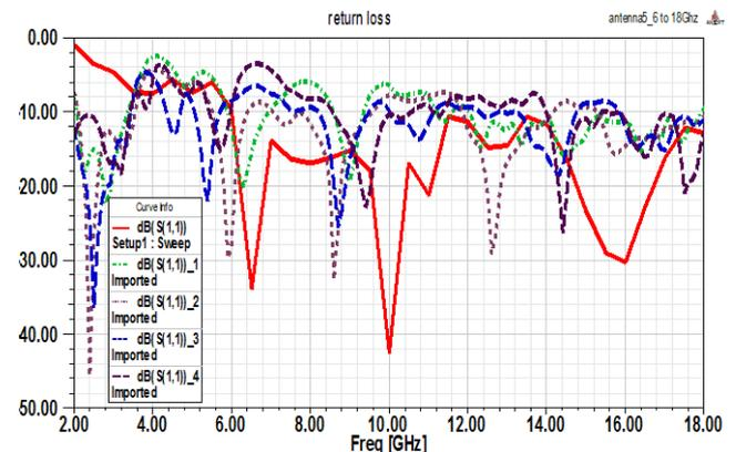
**Fig. 3:** Plot showing return loss enhancement over upper frequency bands through the five stages of evolution
