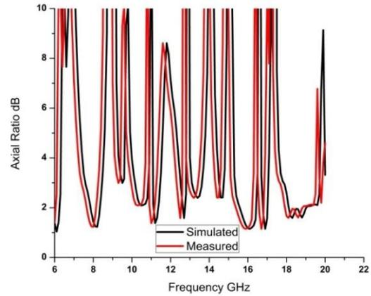
Fig. 8: Axial ratio of the simulated and fabricated antenna.
