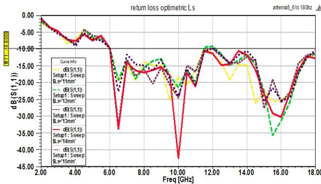
Fig. 6: Stub length tuning from L<sub>s</sub> 11to14mm effect on antenna return loss characteristics
