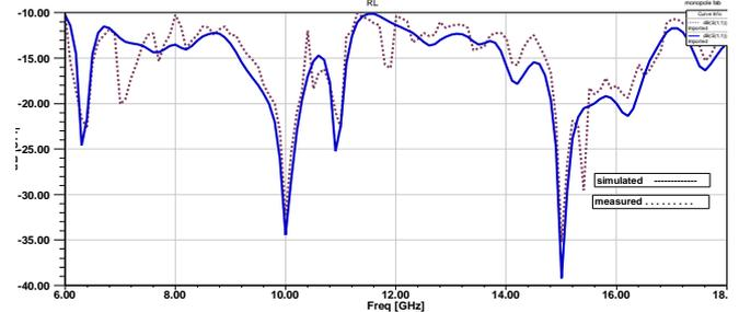
Fig. 7: Return loss plot of the simulated and fabricated antenna.
