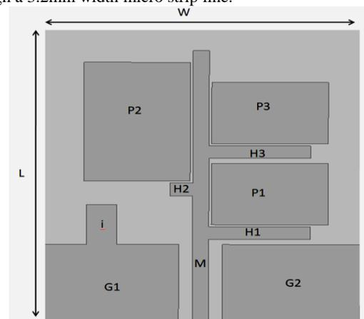
Fig. 1: Multi-octave CPW fed monopole antenna
