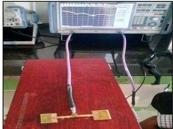
Fig. 16: Testing arrangement of proposed 1X2 Antenna Array using power divider
