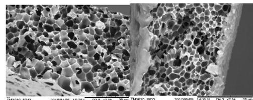
**Fig. 1:** SEM image for surface morphology for pure polysulfone membrane
