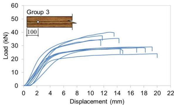
Fig. 2: Typical load versus displacement profiles of ductile behaviour
