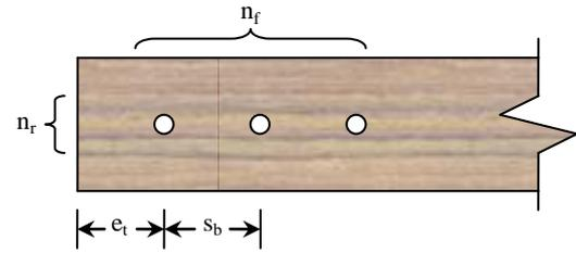
Fig. 1: Variables of timber bolted connections
