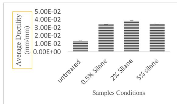
**Fig 5:** Effect of silane treatment on average ductility of rice husk/phenol formaldehyde particleboard
