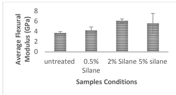
**Fig 4:** Effect of silane treatment on average flexural modulus of rice husk/phenol formaldehyde particleboard
