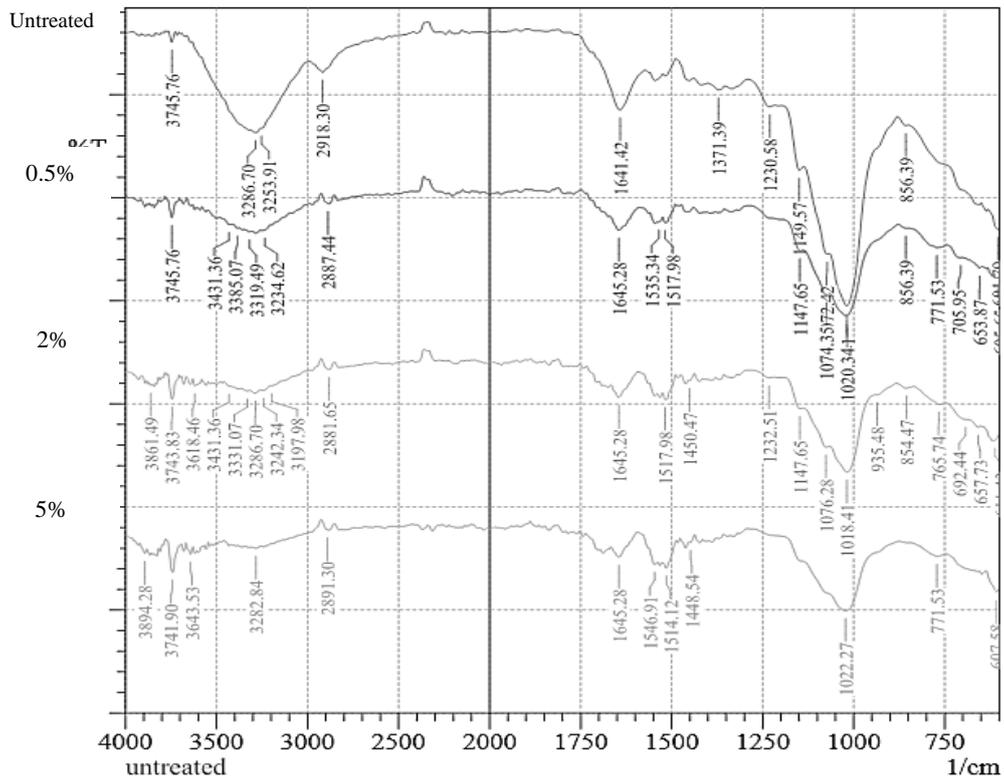
Fig 2: FTIR spectra of untreated and silane treated rice husk
