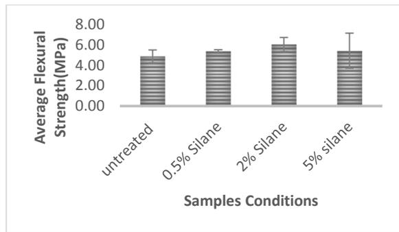
**Fig 3:** Effect of silane treatment on average flexural strength of rice husk/phenol formaldehyde particleboard
