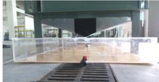
(f) Rainfall simulator recording and monitoring system including ultrasonic sensor device, microcontroller and recording program
