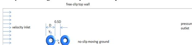
**Fig. 1:** Computational domain in the present study for tandem wheel case (for single wheel case, rear wheel is not included).
