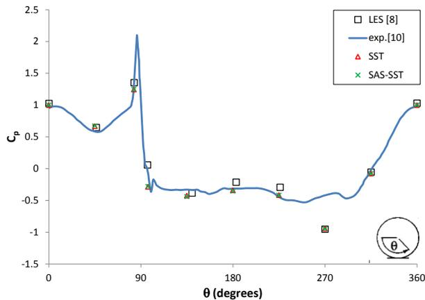
**Fig. 3:** Distribution of surface pressure coefficient at centerline of single wheel in comparison to experimental results [10] and LES results [8]. Position angle around wheel is defined per inset legend courtesy of McManus & Zhang [5].
