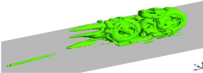
Fig. 5: Vortical structures in a rotating tandem wheel case based on a constant  $\lambda_2$ -criterion.
