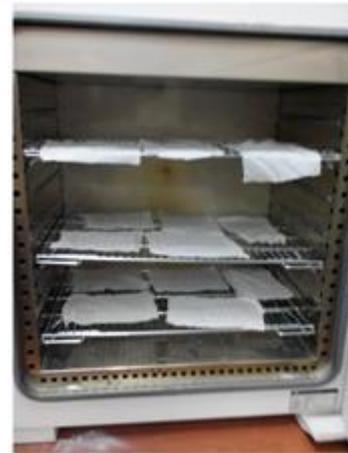
Fig. 3: Treatment of silk fibre with silane coupling agent and ethanol inside an oven.
