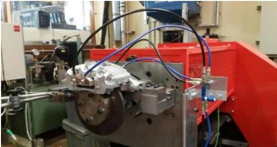
**Fig. 11:** The brake assembly setup used for drag brake testing procedures.
