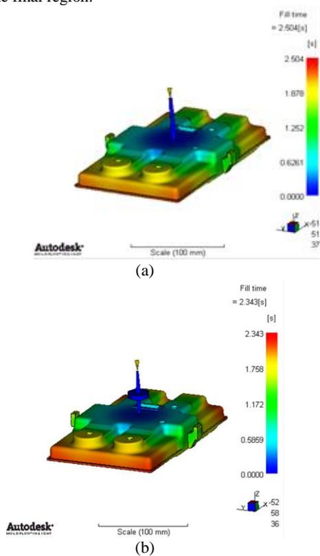
Fig. 7: Filling time of CBT: (a) using a direct sprue gate with a diameter of 6.2 mm, and (b) using a pinpoint gate with a diameter of 1.8 mm.
