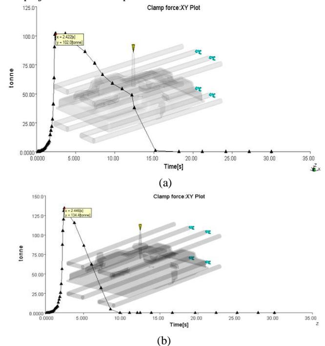
Fig. 9: Clamping force for the two different gates: (a) Direct sprue gate, and (b) Pinpoint gate
