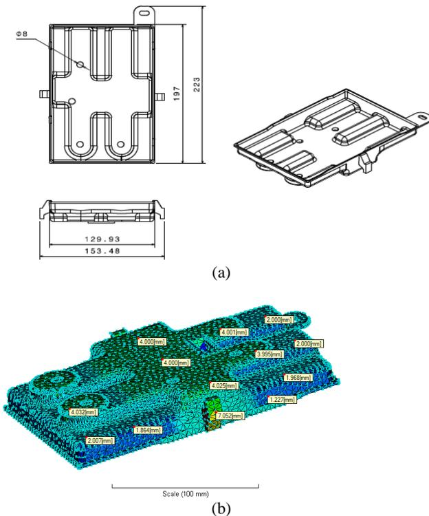
**Fig. 1:** Product appearance. (a) Dimensions of car battery tray, (b) Checking of variable wall thickness in Moldflow
