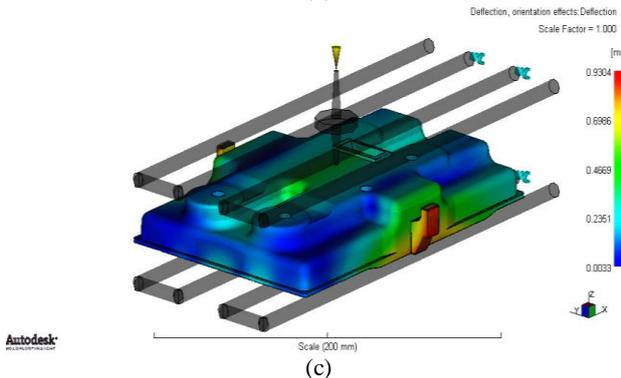
**Fig. 13:** Factors influencing the warpage of the product for the pinpoint gate. (a) Deflection, differential shrinkage, (b) Deflection, differential cooling, and (c) Deflection, differential orientation.
