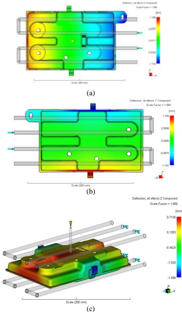
**Fig. 10:** Deflection in warpage analysis for the direct sprue gate in the (a) X-direction, (b) Y-direction, and (c) Z-direction.
