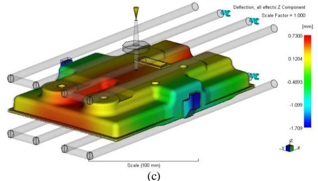
**Fig. 11:** Deflection in warpage analysis for the pinpoint gate in the (a) X-direction, (b) Y-direction, and (c) Z-direction.
