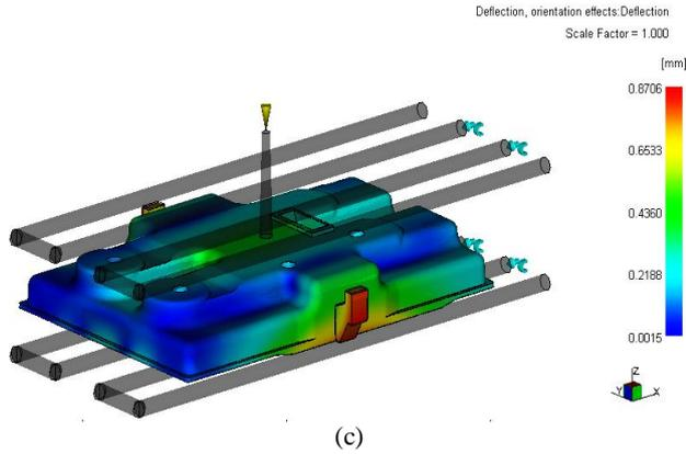
**Fig. 12:** Factors influencing the warpage of the product for the direct sprue gate. (a) Deflection, differential shrinkage, (b) Deflection, differential cooling, and (c) Deflection, differential orientation.
