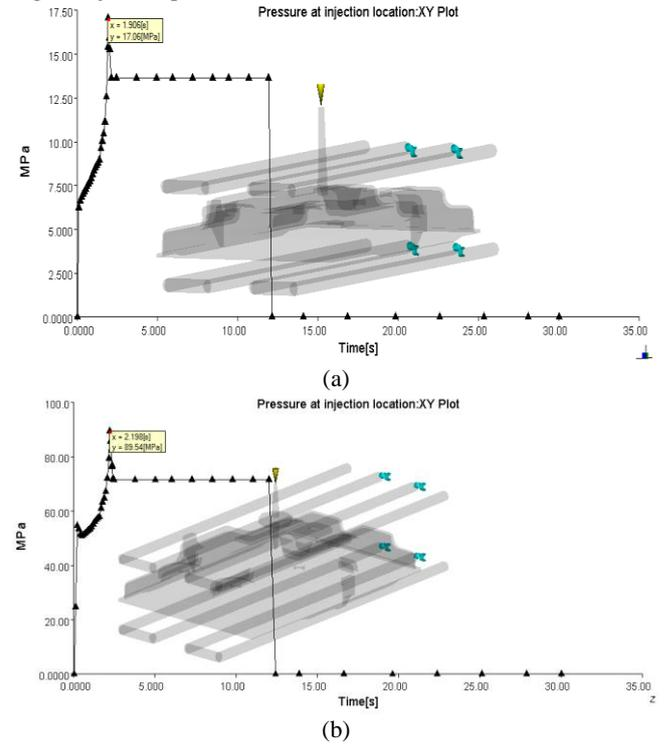
Fig. 8: Injection pressure for the two different gates: (a) Direct sprue gate, and (b) Pinpoint gate
