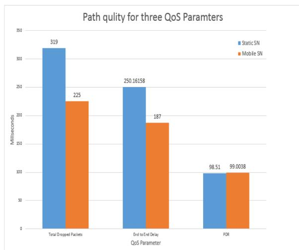
**Fig. 5:** The Network Performance is Improved when Using Mobile SN Because It Gives Lowest Delay Value and Total Dropped Packets in Compare with Using Static SN.
