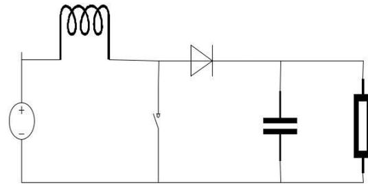
Fig.2: Boost Converter Equivalent Circuit
