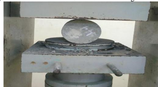
**Fig. 2:** Splitting tensile strength test setup
