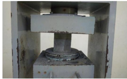
**Fig. 1:** Compressive strength test setup
