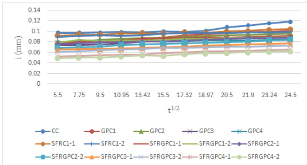
Fig. 2: Sorptivity Test Results
