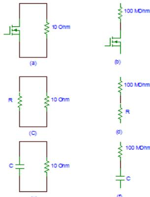
**Fig. 1:** Fault models (a) MOSFET stuck short (b) MOSFET stuck open (c) Resistor stuck short (d) Resistor Stuck open (e) Capacitor stuck short (f) Capacitor stuck open
