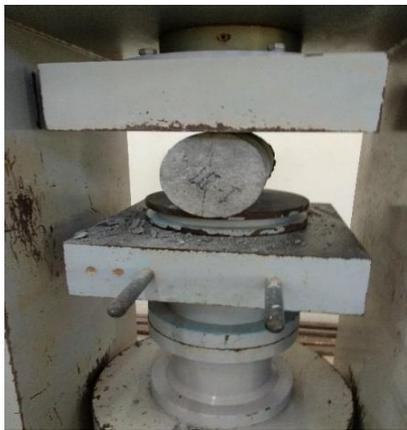
Fig. 4: Split tensile strength test
