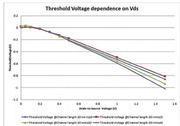
Fig. 4: Threshold Voltage Dependence on thickness of Si film for effective channel length 30nm and  $t_s$  15,20,30,40 nm
