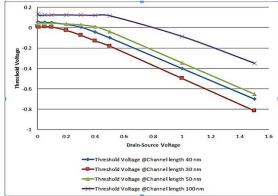
Fig. 3: Threshold Voltage variation for varying channel length
