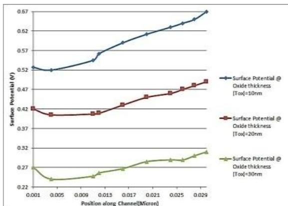
Fig. 2: Channel potential variation with normalized position along the channel length at  $V_{ds} = 0.5 V$
