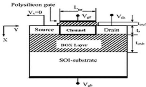
Fig. 1: Cross Section View (x-y) of FDSOI MOSFET
