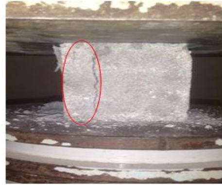
Fig. 7: (a) Failure pattern of 28 days water curing (b) Failure pattern of lime curing
