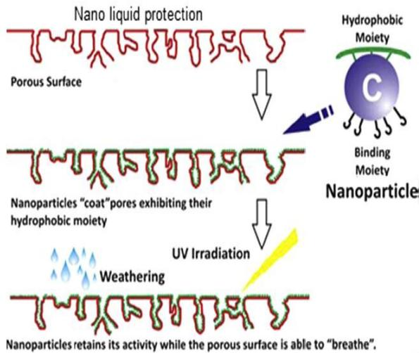
Fig. 1: Performance of nano-liquid on the mortar surface
