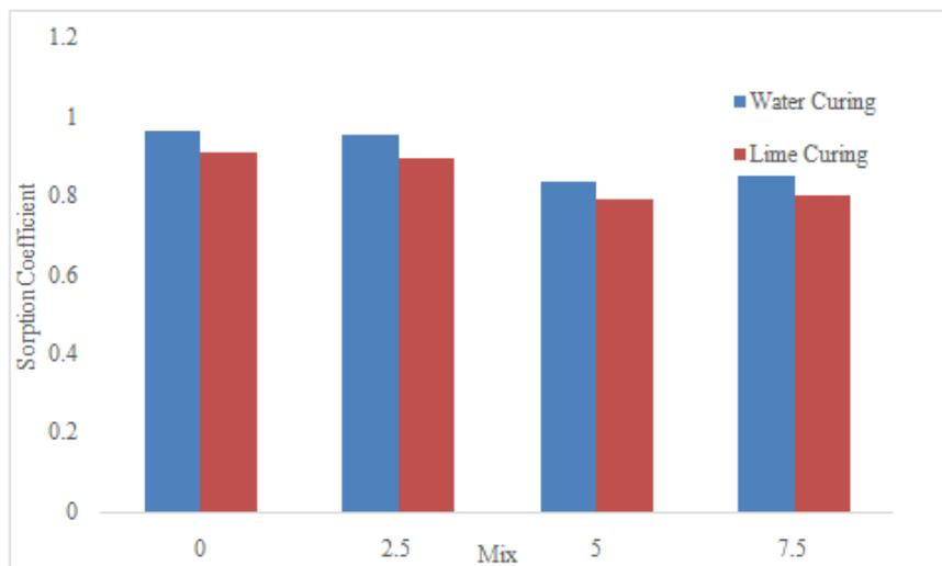
Fig. 8: Sorption coefficients for water and Lime curing
