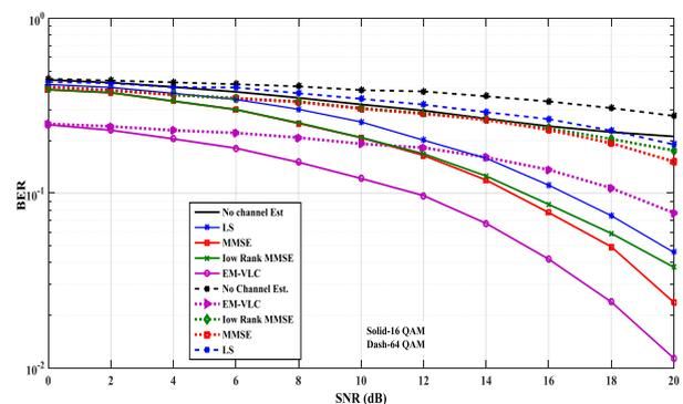
Fig. 7: Comparative BER Performance with 16 QAM and 64 QAM.
