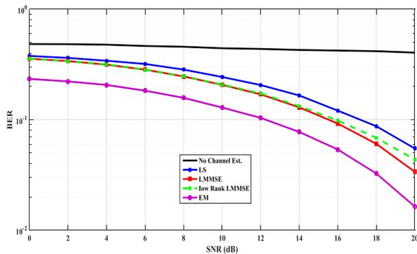
Fig. 4: Comparative BER Performance for 64 FFT and Pilot Spacing of [4].
