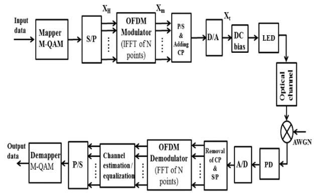
Fig. 1: Block Diagram of DCO-OFDM VLC System.
