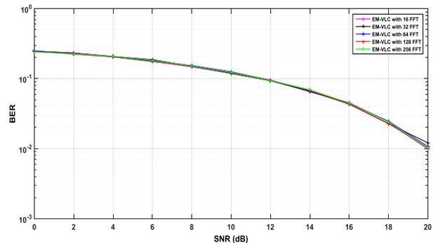
Fig. 6: BER of EM-VLC Algorithm with 64 QAM at Different FFT.
