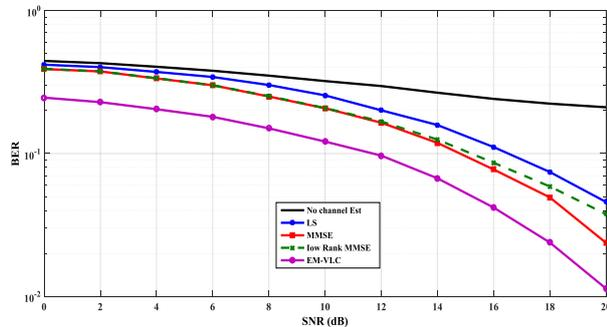
Fig. 3: Comparative BER Performance for 64 FFT and Pilot Spacing of [6].
