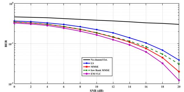
**Fig. 2:** BER Performance of EM-VLC Algorithm for 64 FFT and Pilot Spacing of [8].
