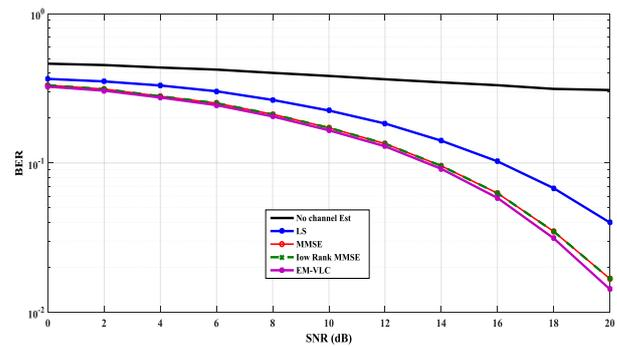
Fig. 5: Comparative BER Performance for 512 FFT and Pilot Spacing of [4].
