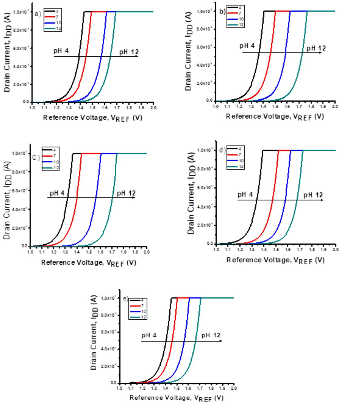
**Fig. 3:** Transfer curve characteristic for ZnO nanostructures at a) deposited-sample, b) 200, c) 300, d) 400 and d) 500 °C post-annealing treatment temperature
