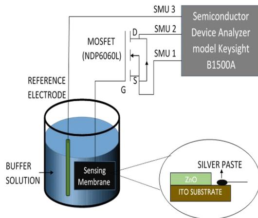
**Fig. 1:** EGFET pH sensing setup using semiconductor device analyzer (Keysight, B1500A)
