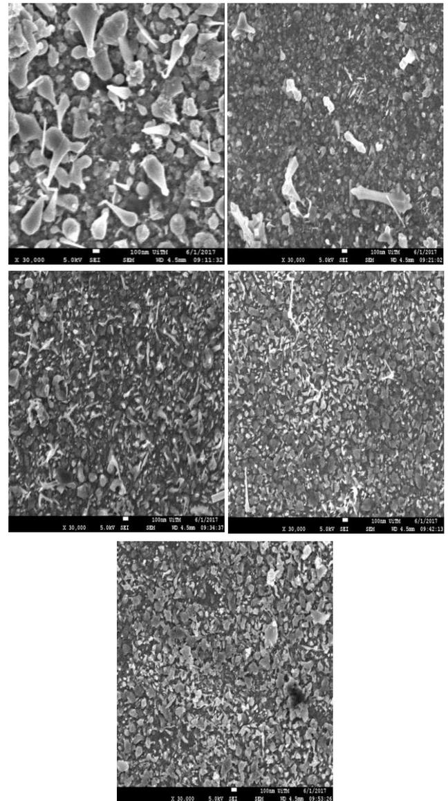
**Fig. 2:** FESEM images of ZnO nanostructures at b) 200, c) 300, c) 400 and d) 500 °C post-annealing temperature using TCVD while a) as-deposited sample
