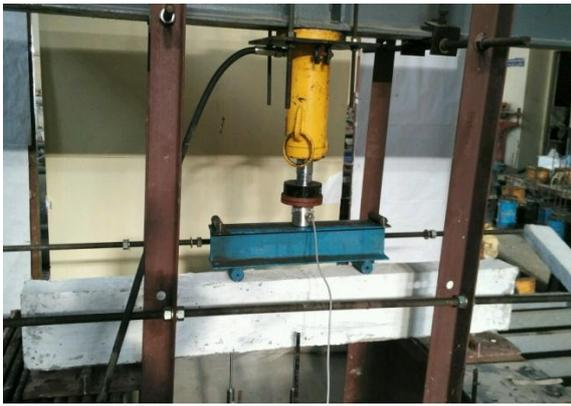
Fig. 2: Experimental setup for testing beams
