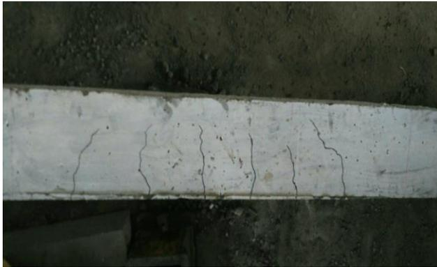
**Fig. 6:** Cracking pattern of beams
