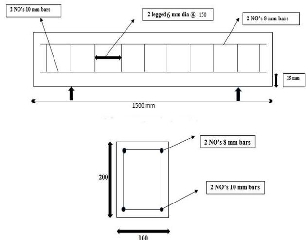
**Fig. 1: Reinforcement details of beam**
