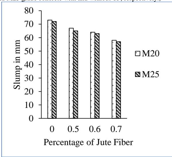
Fig. 3: Slump versus percentage of fiber content
