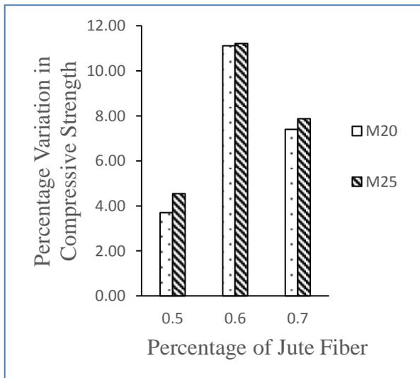
Fig. 4: Percentage variation in compressive strength and fiber content
